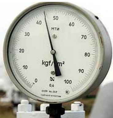
Gas Pressure Gauge
